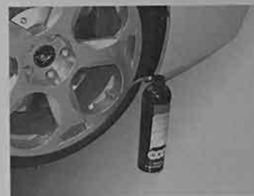
Fig. 118 Tire inflation by the emergency inflator
