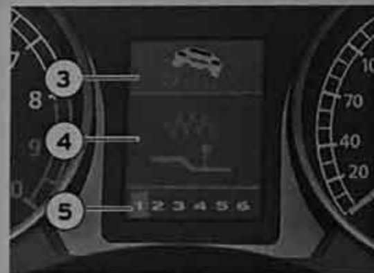
Fig. 74c Eogear controls and displays: slippery roads display in case of eogear failure
