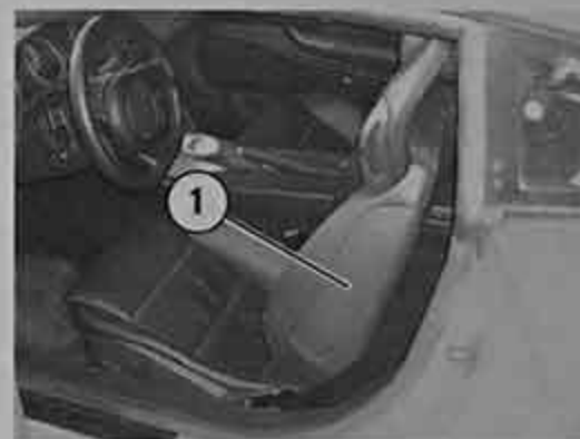
Fig. 91 Location of side airbag in driver's seat
