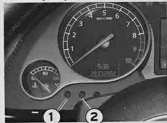
Fig. 38 Instrument lighting controls
