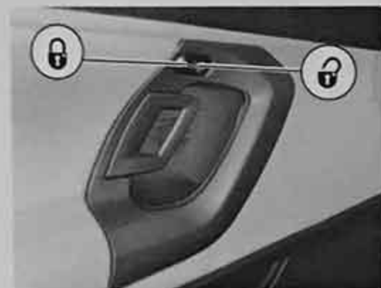
Fig. 30 Driver's door: central locking switch
