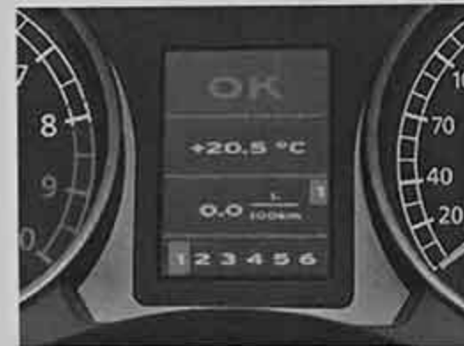
Fig. 21 On-board computer display: current fuel consumption
