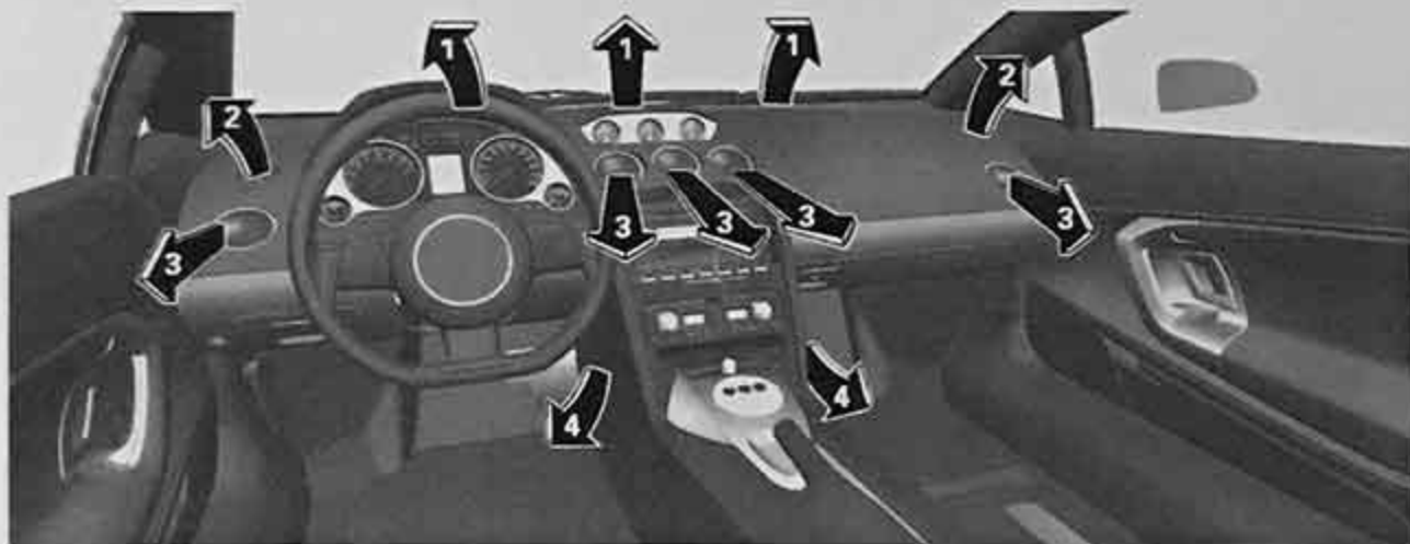
Fig. 70 Dashboard: air vents.
