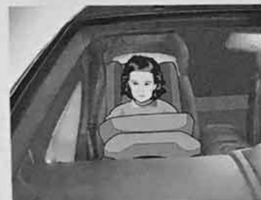
Fig. 96 The child is sitting in a restraint system and is wearing a seat belt
