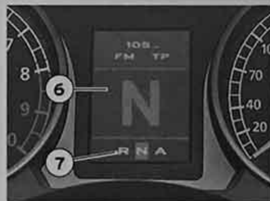
Fig. 74b Eogear controls and displays: gear in neutral position and automatic mode displays
