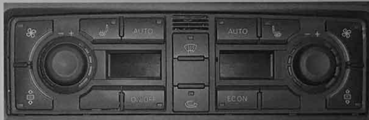
Fig. 65 Air conditioning system controls
