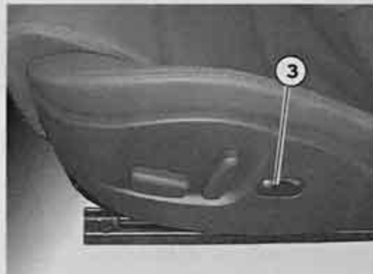
Fig. 57 Lumbar support power adjustment control
