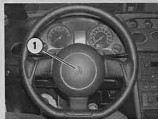
Fig. 87 Driver's airbag in the steering wheel
