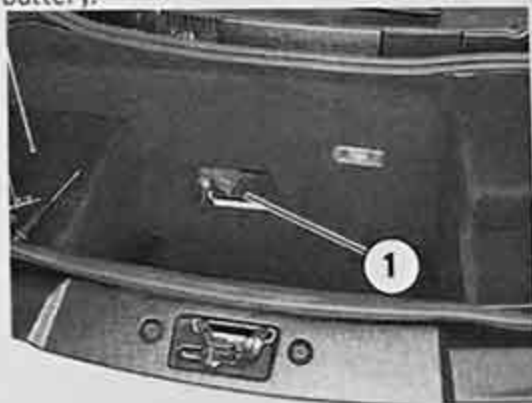
Fig. 119 Accessing the battery cables
