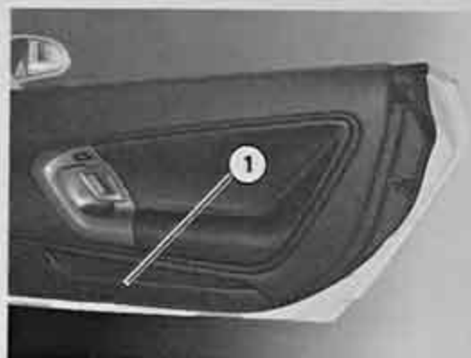
Fig. 63 Door trim storage compartment detail
