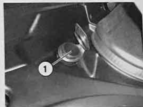
Fig. 114 Luggage compartment: windshield washer container filler pipe.
